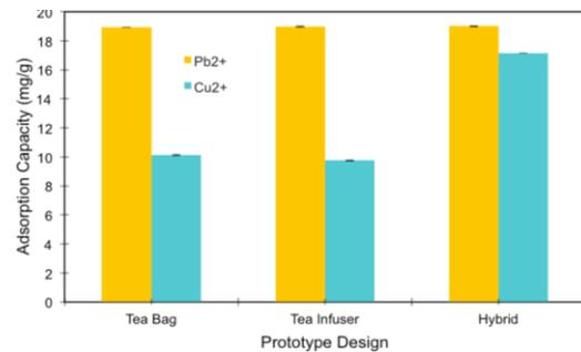
Figure 7 Bar graph showing the effect of prototype design on the adsorption of  $Pb^{2+}$  and  $Cu^{2+}$  ions. Error bars represent standard deviation for technical triplets.
