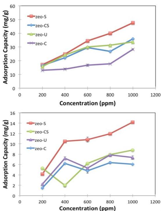
Figure 5 Effect of concentration and varying treatment of zeolite on removal of  $Pb^{2+}$  ions (left) and  $Cu^{2+}$  ions (right) in 2h. Error bars represent standard deviation for technical triplets.
