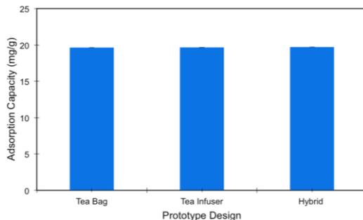
Figure 6 Bar graph showing the effect of prototype design on the adsorption of MB dye. Error bars represent standard deviation for technical triplets.
