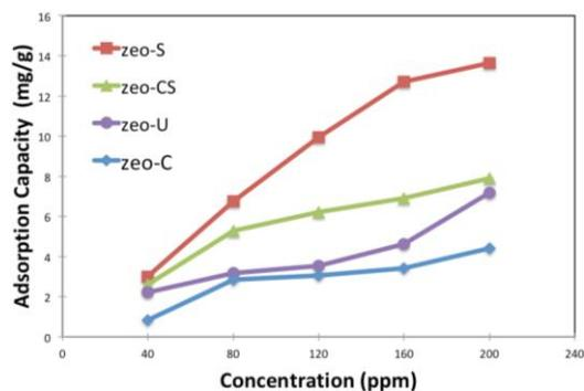
Figure 4 Effect of concentration and varying treatment of zeolite on removal of MB dye in 2h. Error bars represent standard deviation for technical triplets.
